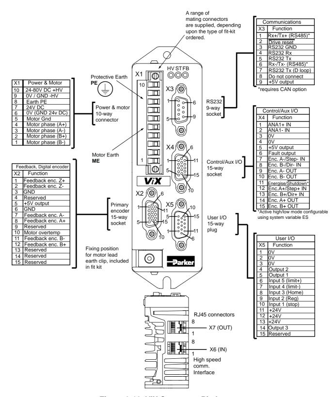
Figure 3-10. ViX Connector Pin Layout
